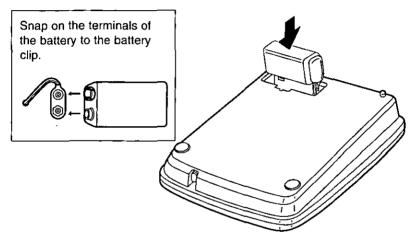
• If "Lo" flashes for over 10 seconds after installing a new battery, disconnect the AC adaptor and reinsert it again without removing the battery. It will disappear after 10 seconds.
