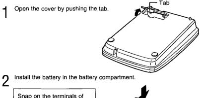
Snap on the terminals of the battery to the battery clip.
